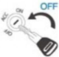
Switch off the engine and keep sparks, flames, cigarettes away from battery at all times before removing the old battery.
