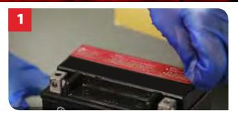
1. Remove foil strip which runs across the top of the battery filling reservoir.
