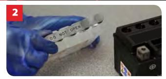
2. Remove electrolyte from safety bag and remove strip of caps. **IMPORTANT:** Do not discard this strip as it acts as the battery sealing plug and is required later. Do not attempt to separate the individual electrolyte cells.
