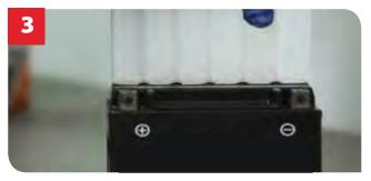
3. Place electrolyte container, sealed top of the cells down, into the filler ports of the battery and push down to break the seals. Ensure the electrolyte container is kept in an upright position during this process.
