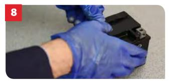
8. After charging is complete, press the cap strip firmly into the cap seats. It will click when correctly in place. Do not pound or hammer into place. IMPORTANT: Never remove the cap strip or add water or electrolyte to the battery during its service life.
