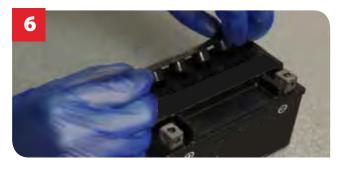
6. Loosely replace the cap strip (as referred to in step 2) over the filling holes. Do not press down firmly or lock this into position at this stage.
